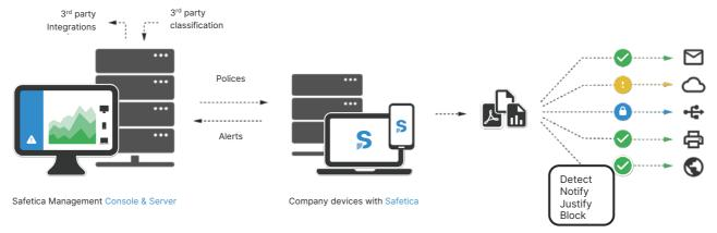
The physical or virtual server runs a database with endpoint activity and security records. The Safetica Management Console enables admins to manage security policies and display the collected information.
